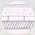
MADRAS ROOF TREATMENT
